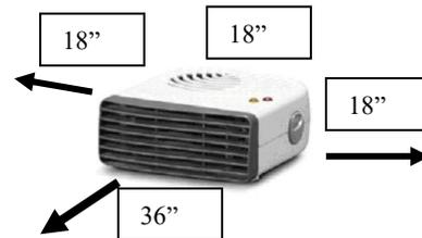
4. One common location for smaller personal electric heaters is under desks. This is a potentially hazardous place for them. It is difficult to maintain proper clearances. Paper and other highly combustible material can accidentally fall or be kicked into the clearance area around the heater. Also, many of these heaters are not approved for use on carpet.
